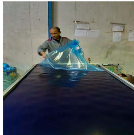
*Figure 110 Absorber assembly [3]*
