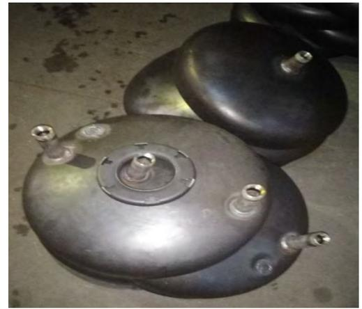
*Figure 53 Welded pipe connections [3]*
