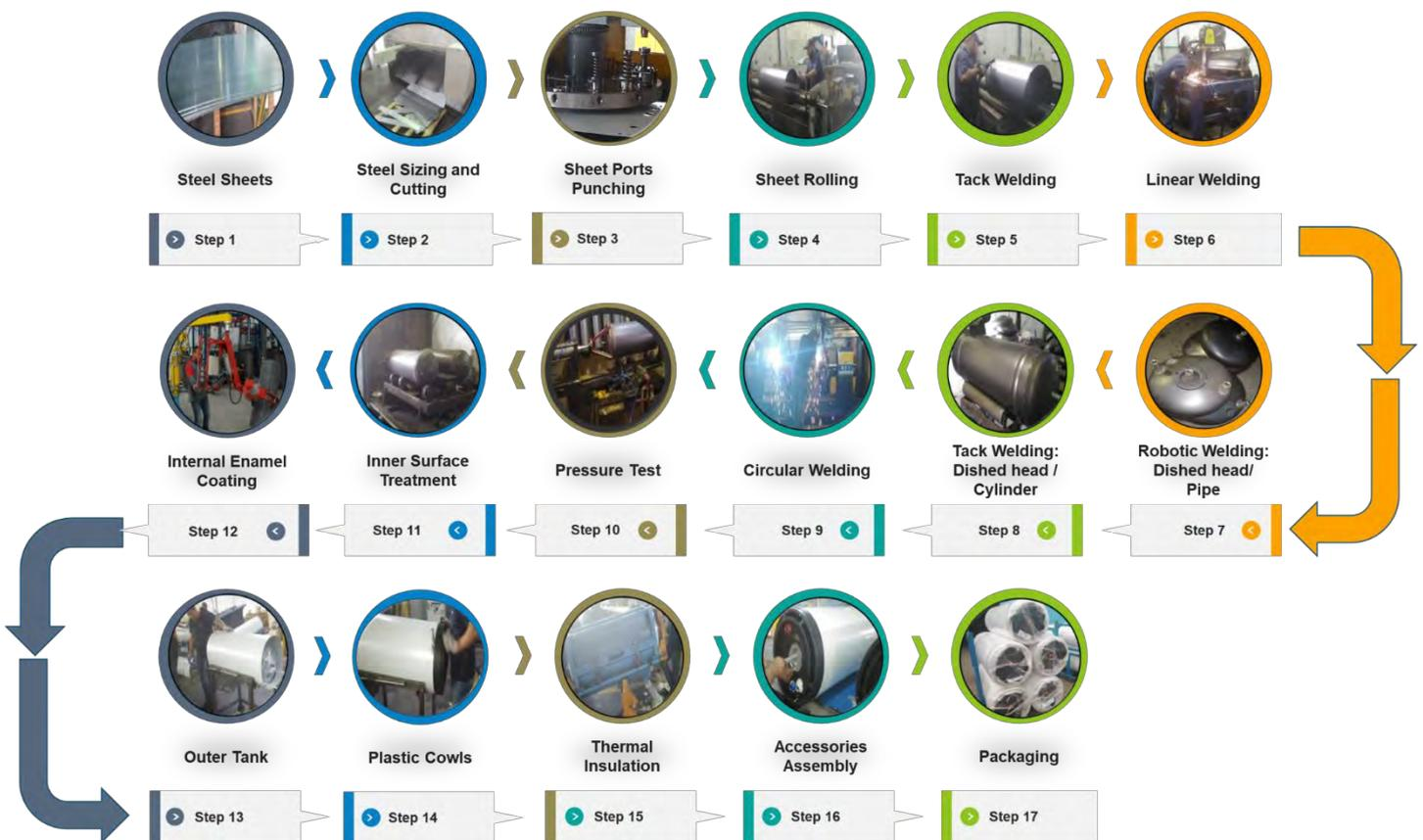
Figure 40 Flow chart of storage tank manufacturing process
