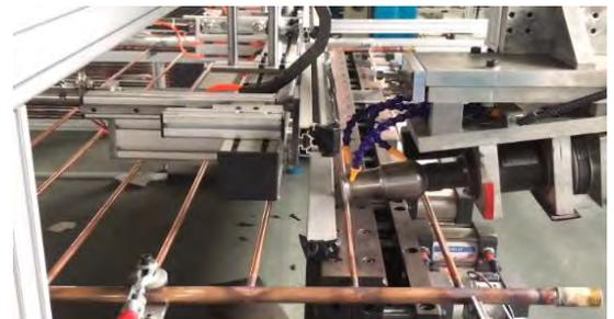
Figure 102 Example setup of the roughen treatment process [4]
