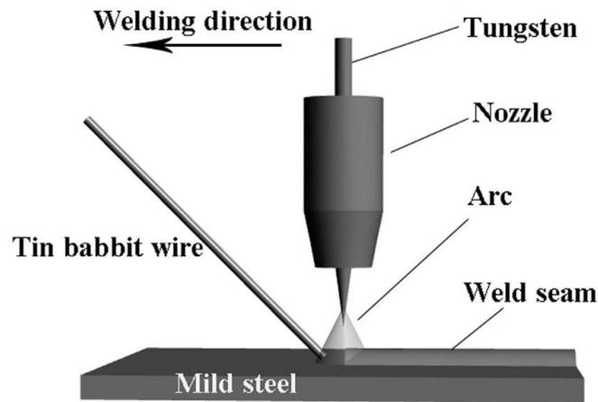
Figure 47 Schematic diagram of arc welding [5]
