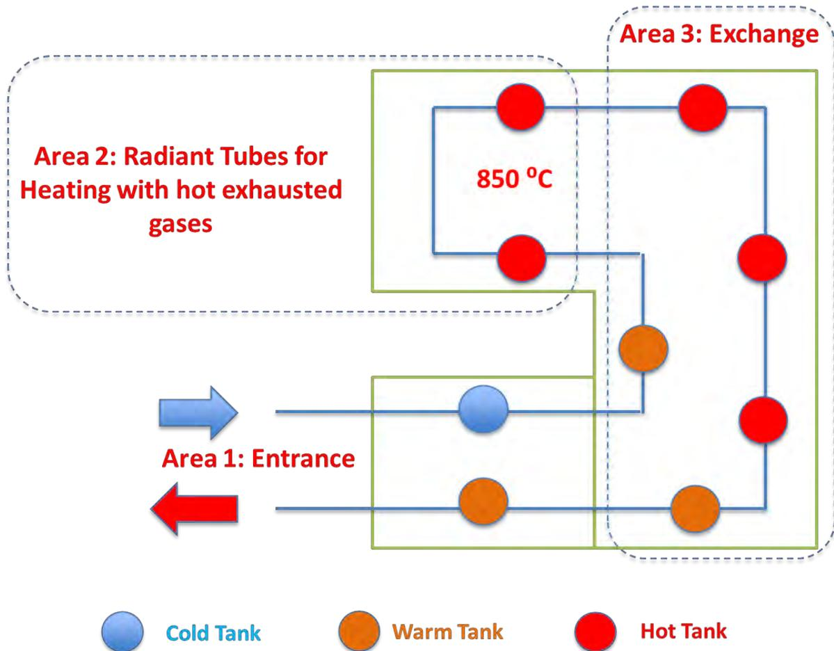
Figure 69 Enamel coating firing process of tanks
