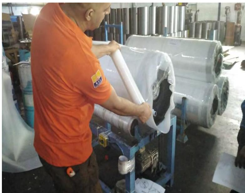
*Figure 83 Packaging of SWH storage tank*
