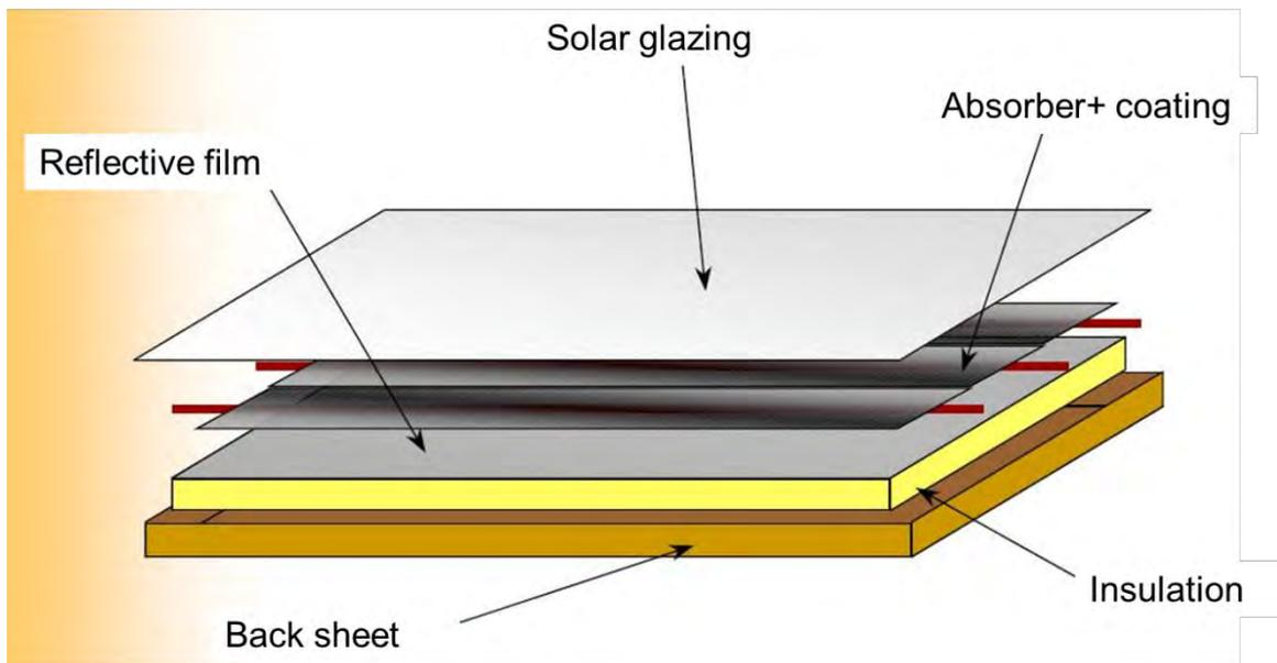
*Figure 90 Flat plate collector main components [3]*
