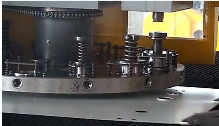
Figure 43 Ports punching in tank body [4]
