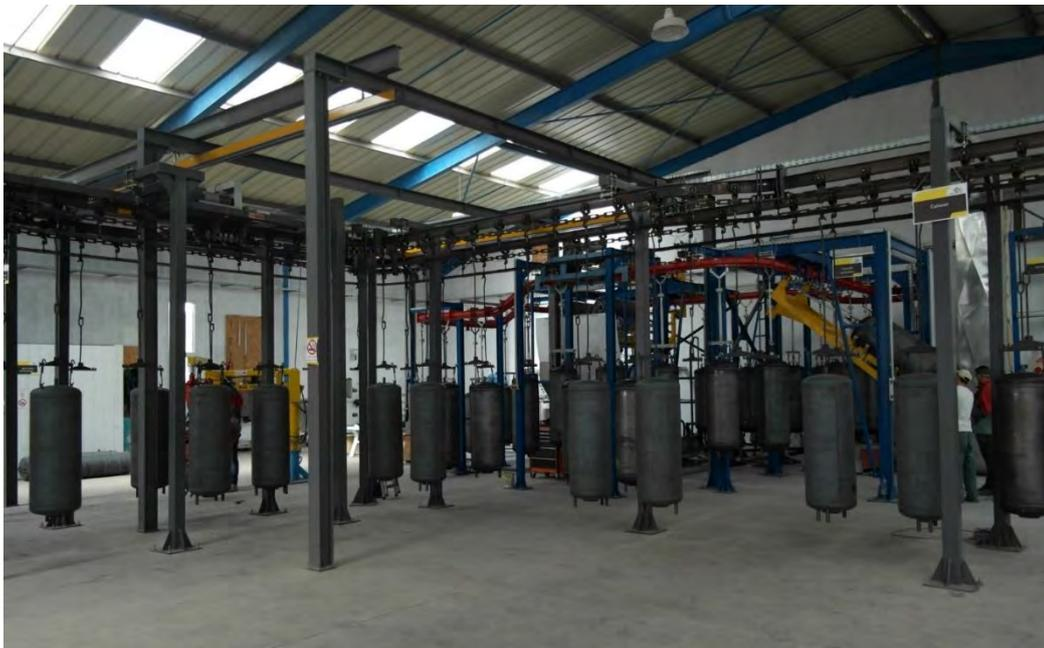
*Figure 71 Enamel coated tanks cooling process [3]*
