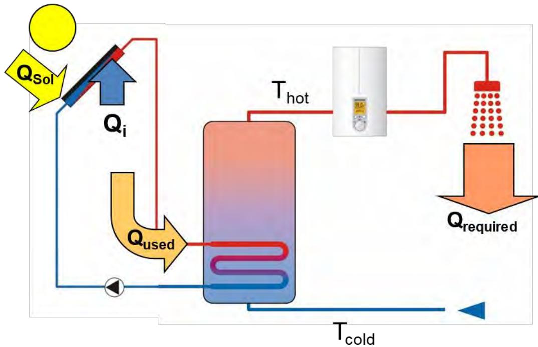
Figure 20 Schematic diagram of SWH system as example
