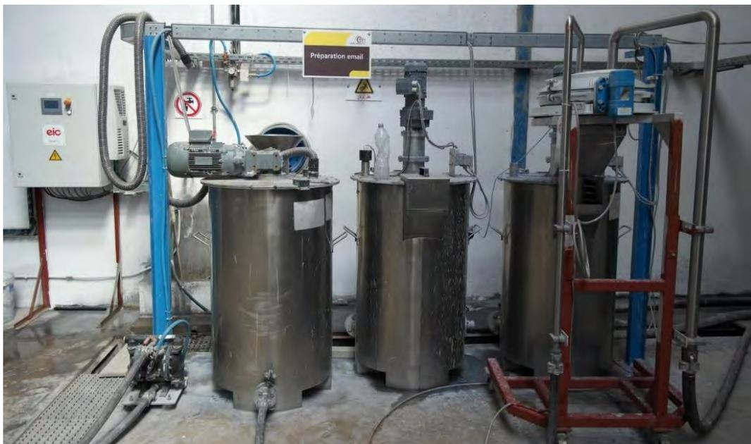
Figure 64 enamel coating preparation mixing unit [3]
