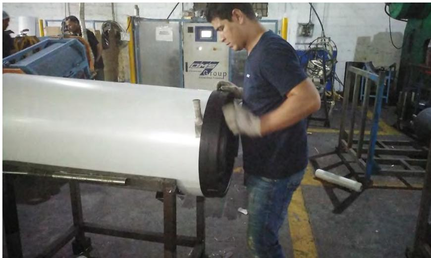
Figure 77 Plastic cowl fixing [3]
