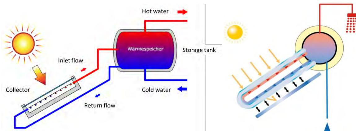
Figure 7 Functional diagram of a Thermosiphon open systems [1]
