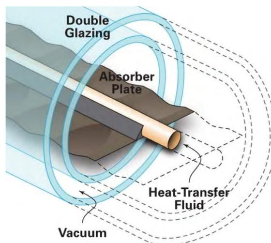
Figure 25 Heat pipe breakdown components
