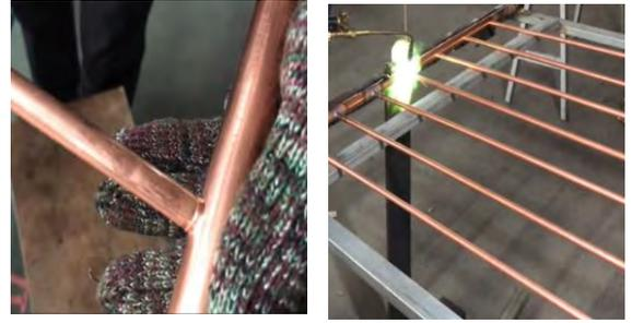
Figure 100 Welding riser tubes with header tube [4]
