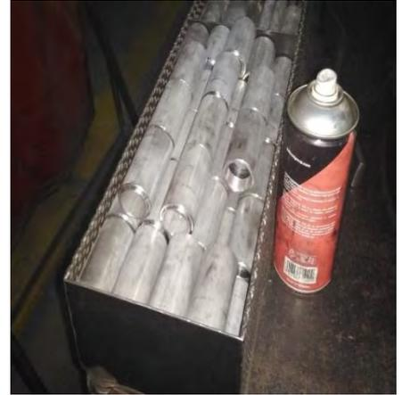
Figure 51 Circular cutting for tank end covers
