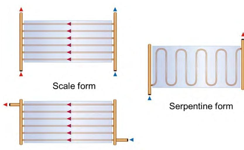
Figure 92 Absorber grid form types [3]
