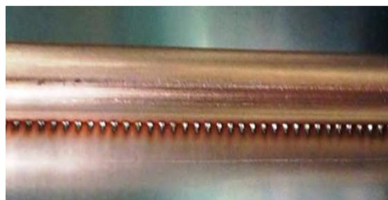
*Figure 105 Laser welding of riser tubes and absorber sheet [4]*
