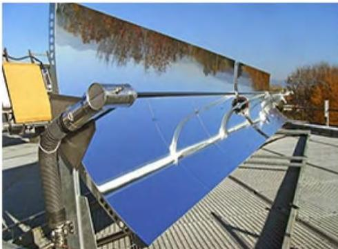
*Figure 15 Parabolic trough collector,
