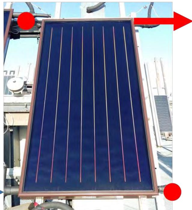
Figure 130 Water flow direction for exposure test (internal shock)
