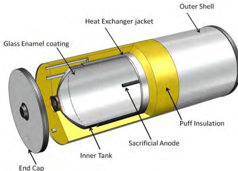
Figure 88 Sample of double jacket storage tank
