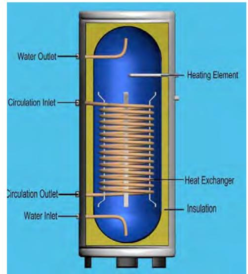
Figure 38 Sample of embedded coil storage tank
