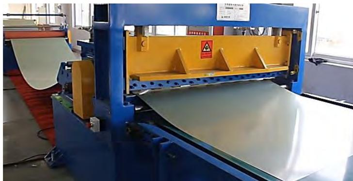
*Figure 42 Inner tank sheet cutting [3]*
