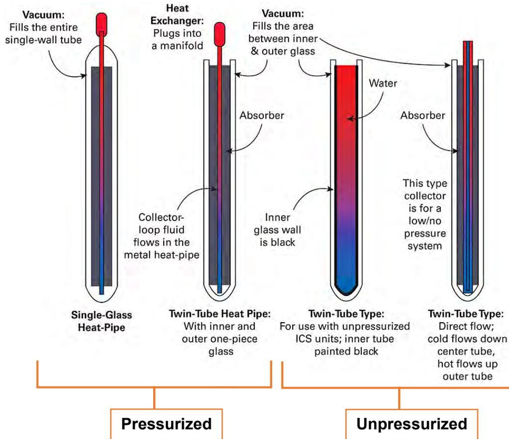
Figure 26 Heat pipe breakdown components
