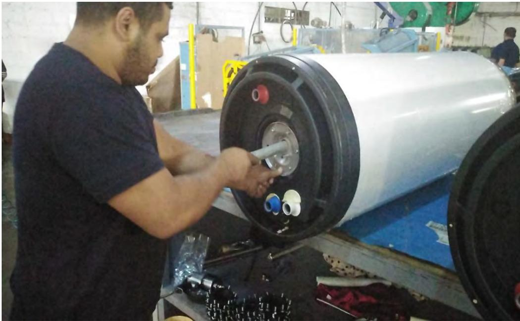
*Figure 81 Mg rod fixing [3]*
