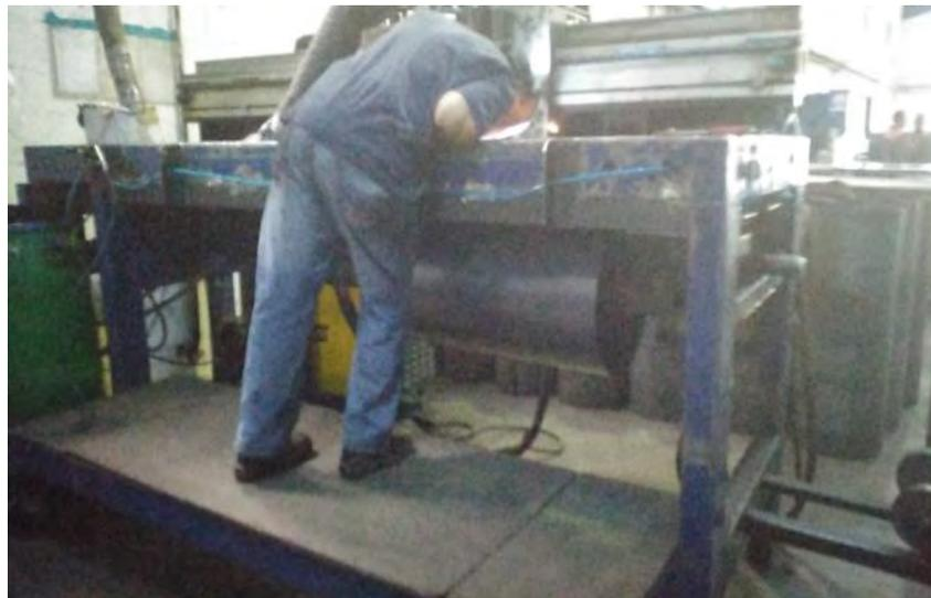
*Figure 46 Linear welding of inner tank [3]*
