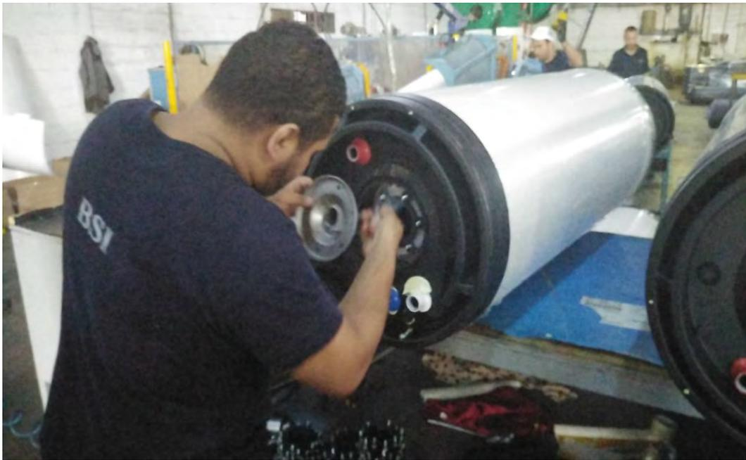
*Figure 80 Barrel (Stainless Steel) fixing [3]*
