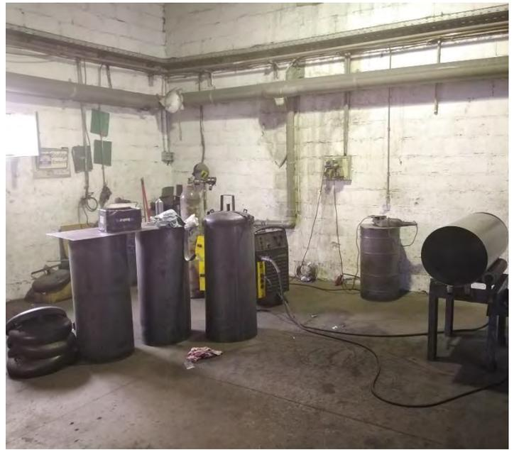
Figure 123 Rolled tanks area and MIG-MAG welding area [3]
