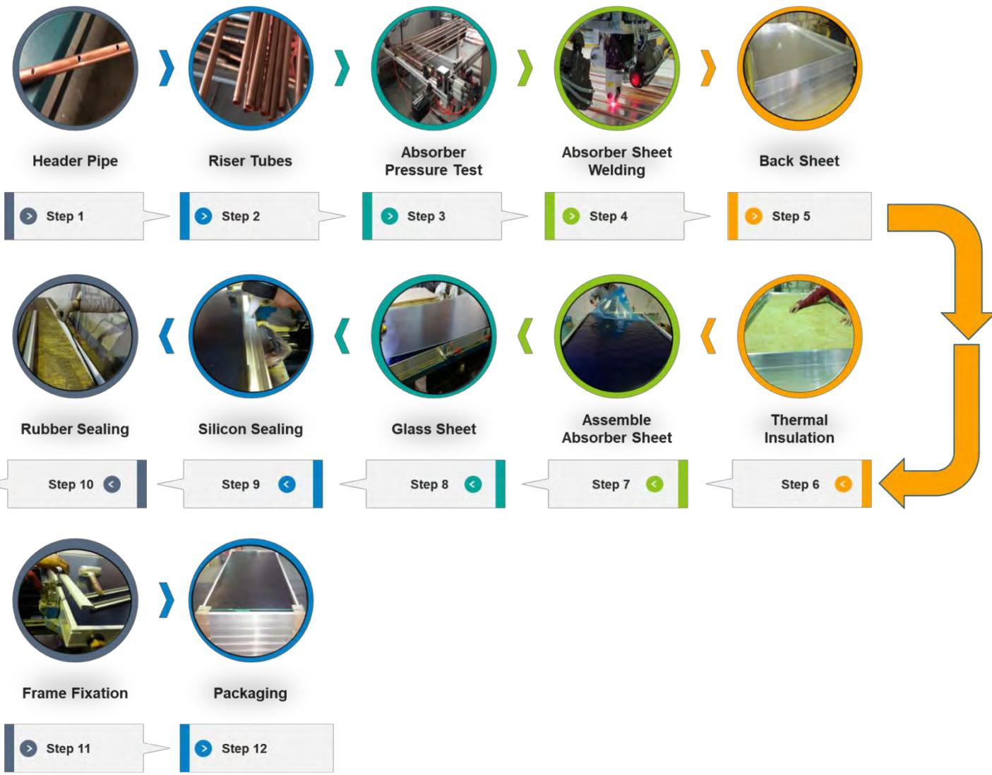
Figure 95 Flow chart of flat plate collector manufacturing process
