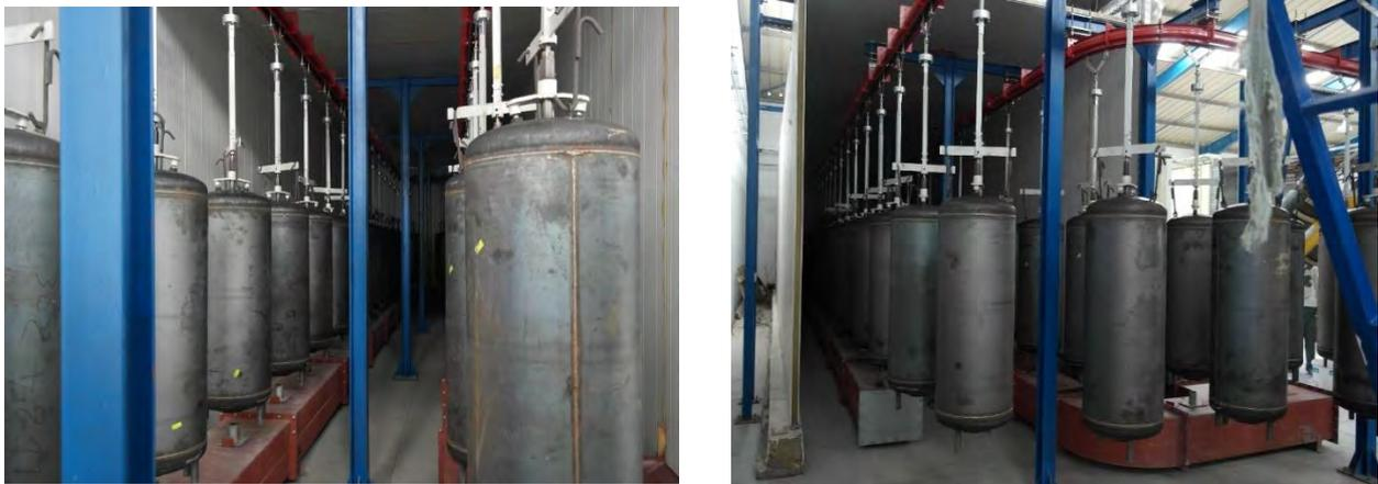
*Figure 66 Tanks drying tunnel process [3]*
