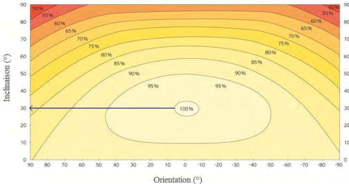
Figure 5 Optimum inclination and orientation angles for Cairo
