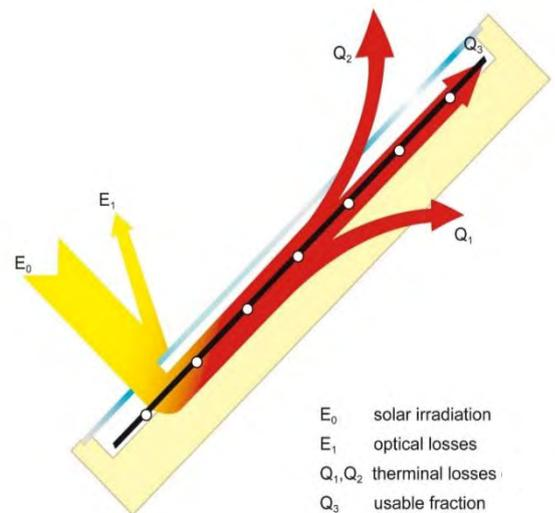
Figure 6 Schematic diagram for absorbed energy in solar collector
