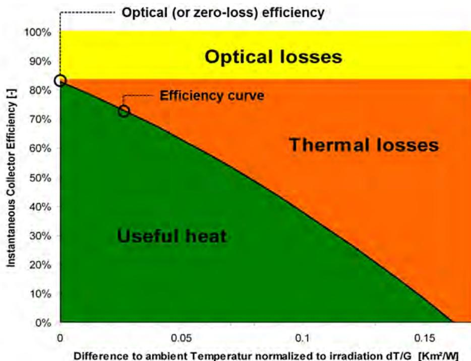
Figure 10 Solar collector efficiency curve
