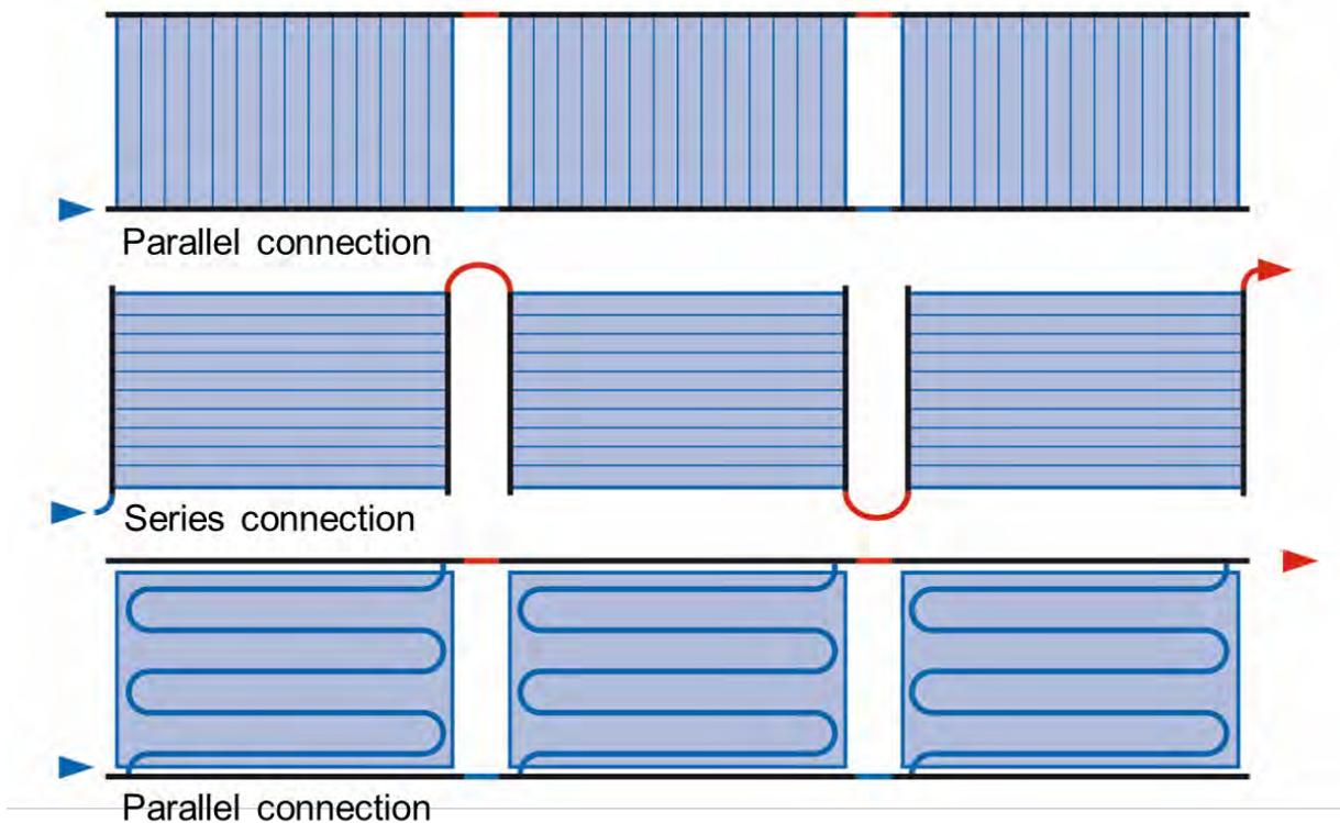
Figure 93 Absorber types of connections [3]
