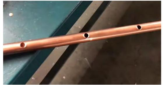
Figure 97 Punched holes along header tube length [4]
