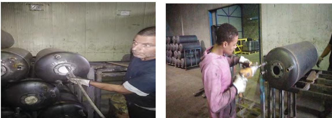
*Figure 63 Visual inspection after blasting process [3]*
