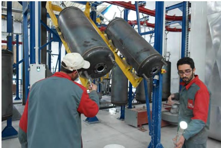
*Figure 74 Visual inspection of internal enamel coating [3]*
