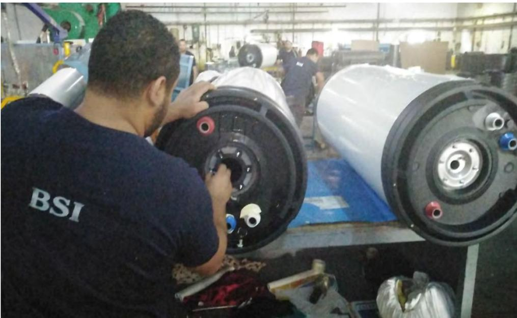
*Figure 79 Seal joint fixing [3]*
