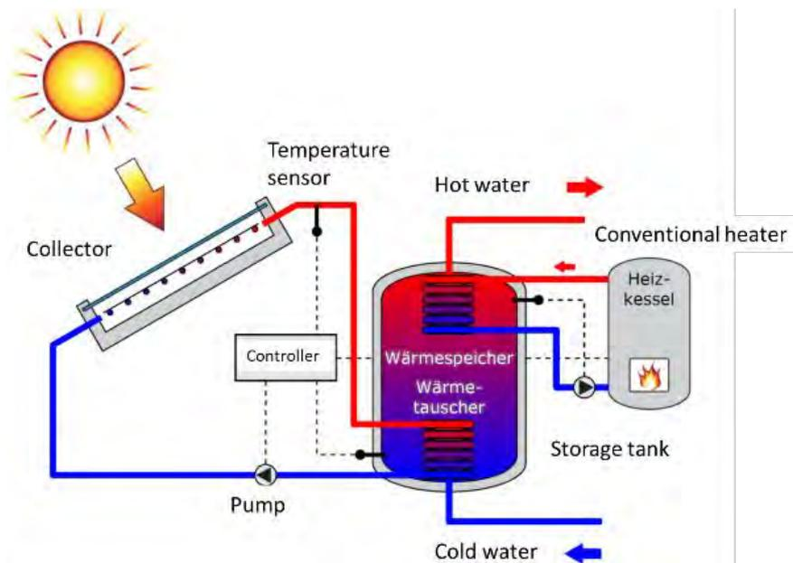
Figure 9 Functional diagram of a forced circulation system [1]
