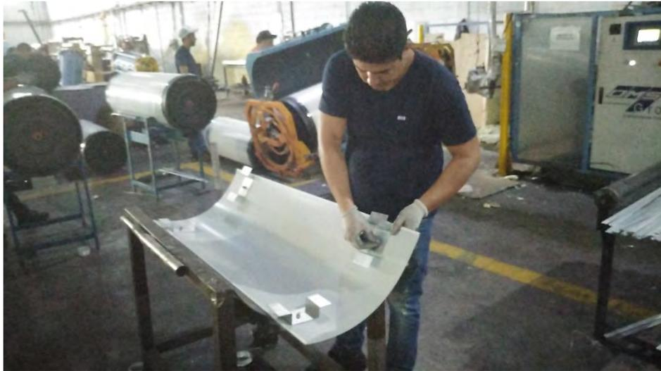
Figure 75 Preparation of the outer tank [3]
