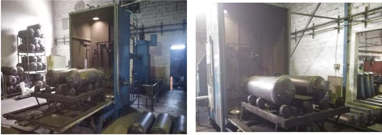
*Figure 62 Inner tank sand blasting process (preparation and loading) [3]*
