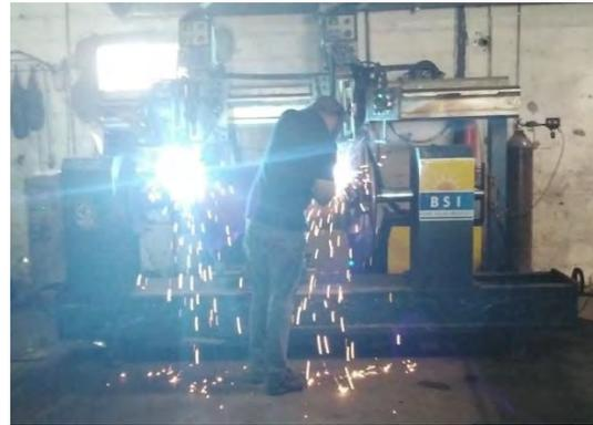
Figure 55 Circular welding using Automatic MIG welding machine [3]
