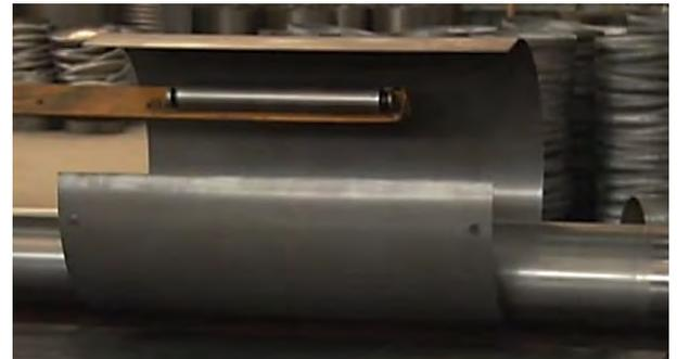
Figure 44 Tank body rolling [4]
