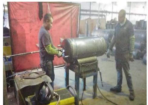
Figure 57 Quality control of circular welding [3]
