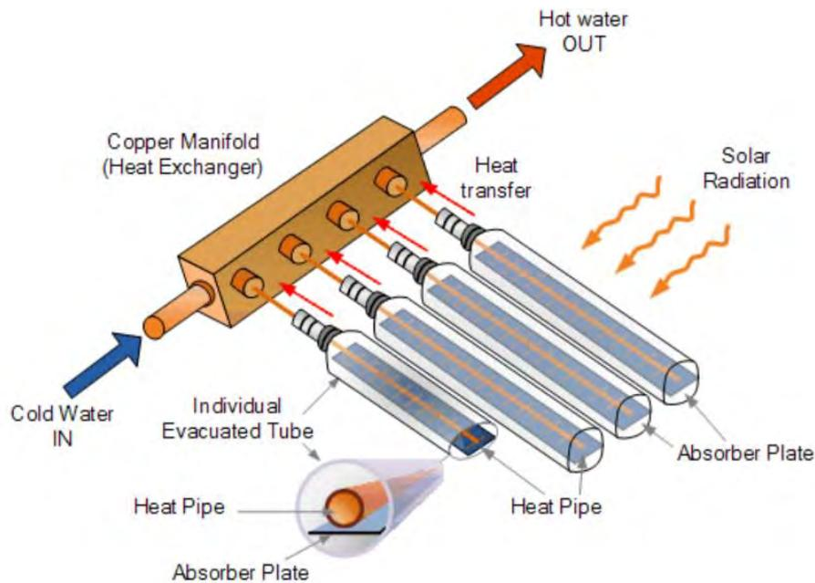
Figure 24 Evacuated tube collector typical breakdown components
