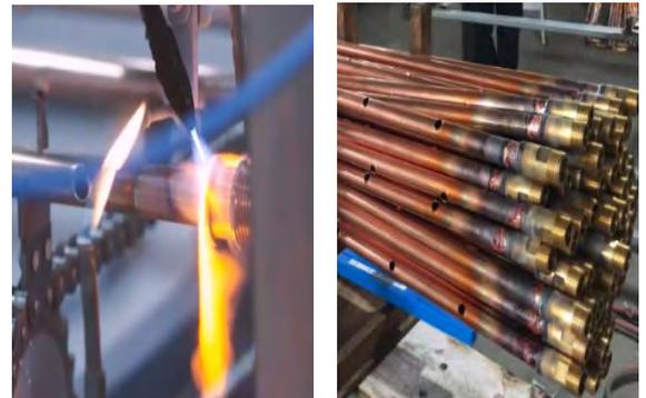
Figure 98 Header tube fitted with connection joints [4]
